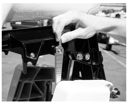
Figure 5.2 Tilt Lock in the Locked Position
