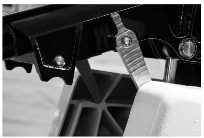
Figure 4.10 – Tilt Lock Engaged
