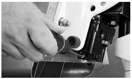
Figure 4.12– Loosening the Release Valve Fastener
