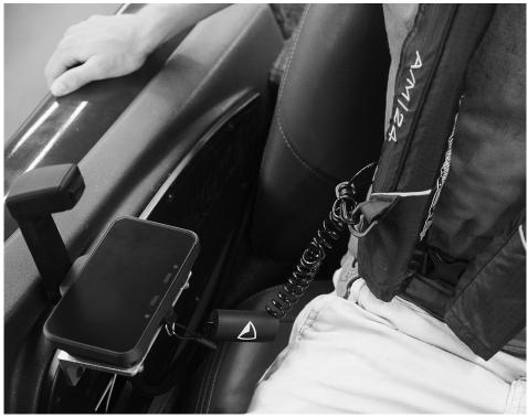
Figure 4.22 – Emergency Stop Connected to the Boat Operator
