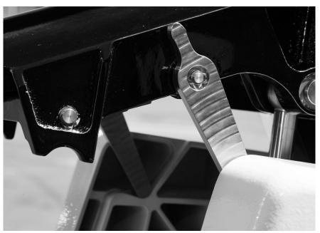
Figure 9.1 – Tilt Lock in the Locked Position
