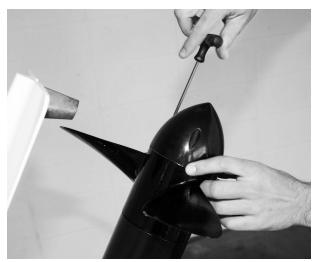
Figure 10.15 – Tightening Tail Cone Fasteners
