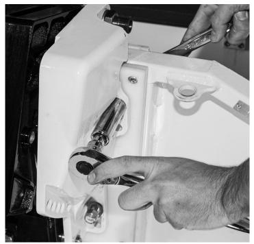
Figure 10.4 – Tightening Bolts with Wrench and Ratchet Extension
