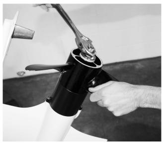
Figure 10.14 – Tightening Propeller Nut
