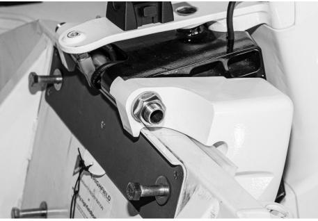
Figure 10.3 – Bolts Aligned in Transom and Outboard
