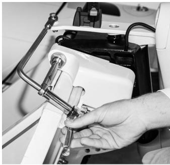
Figure 10.11 – Secure Steering Linkage to Steering Cable
