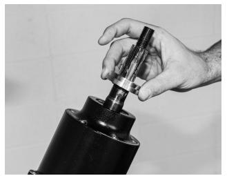
Figure 10.13 – Bow Side Propeller Thrust Washer on Propeller Shaft
