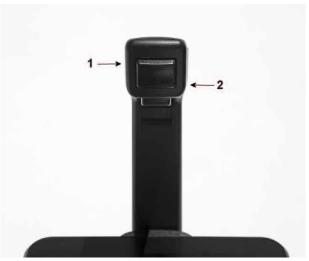
*Figure 4.7 – Tilt/Trim Button on the Throttle*
