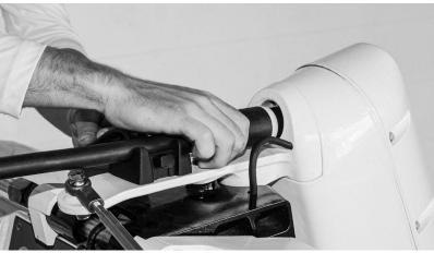
Figure 4.11 – Removing the Cable from the Outboard
