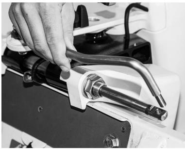
Figure 10.10 – Insert Steering Linkage on Steering Cable Hole
