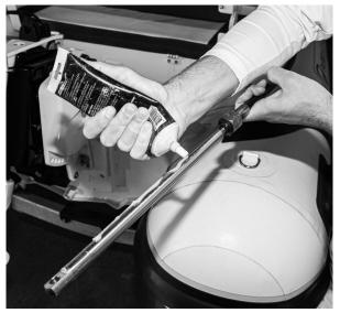
Figure 10.5 – Applying Marine Grease on Steering Cable
