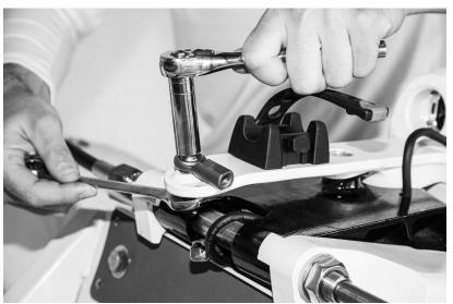
Figure 10.9 – Attaching Steering Linkage to Outboard's Steering Arm
