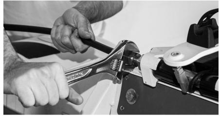
Figure 10.7 – Tighten the Nut on the Steering Tube
