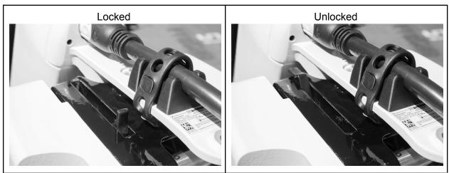
Figure 4.14 – The Steering Lock in the Locked and Unlocked Position
